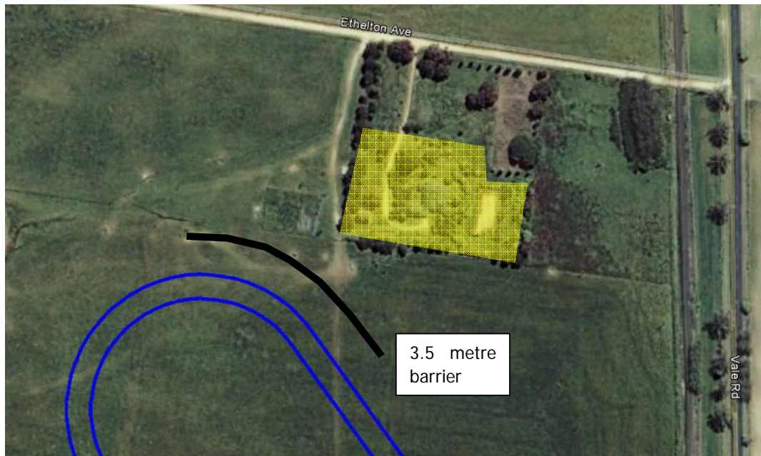
Figure 7-2 Option 2 – Recommended Location of Noise Barrier
