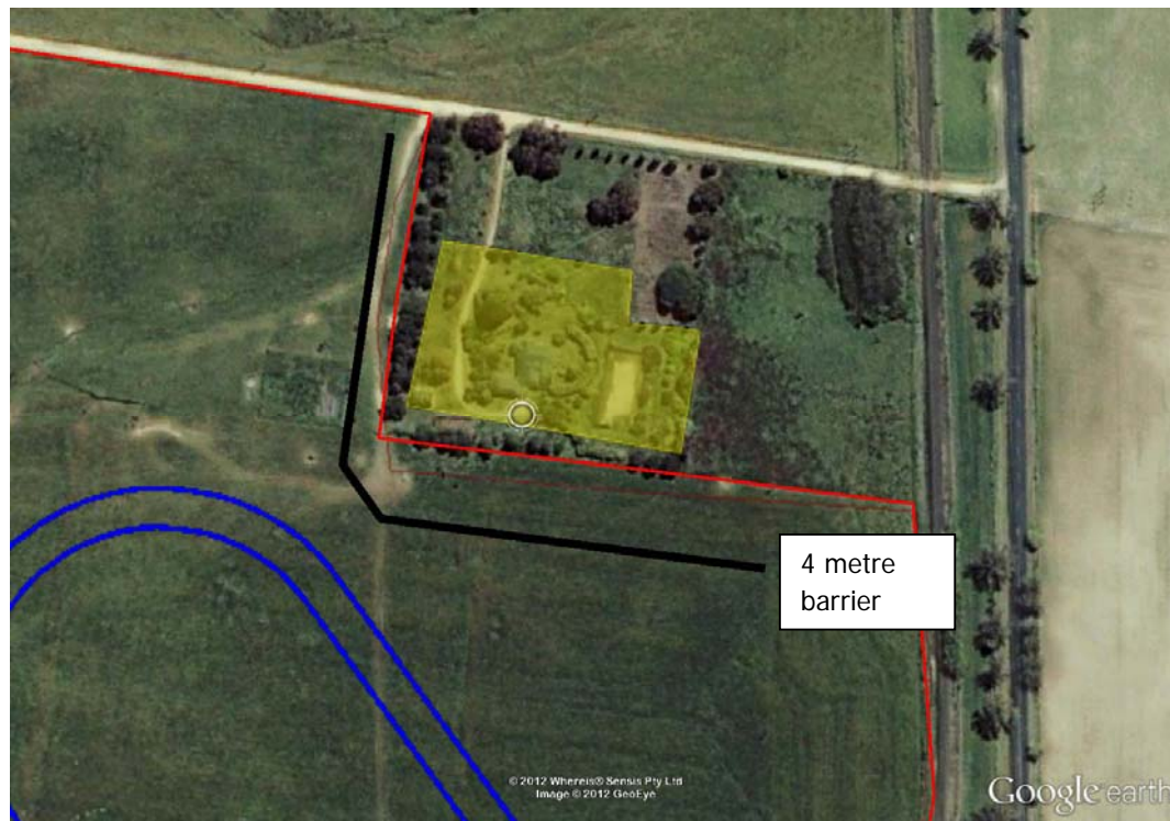
Figure 7-1 Option 1 – Recommended Location of Noise Barrier
